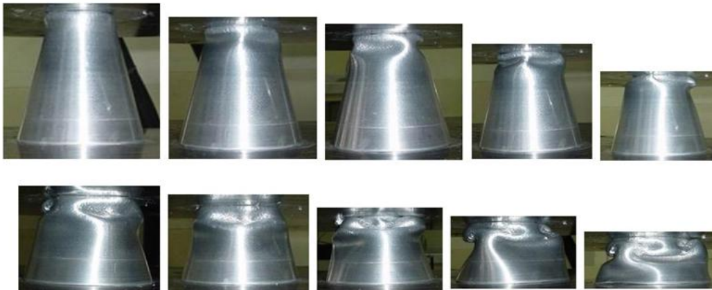
Fig. 5. Typical deformation history of conical shells under axial compression.
