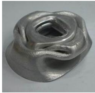
Fig. 4. Typical deformed specimens (a) cylindrical shell with varying thickness along the length (b) conical shells with varying thickness along the length.
