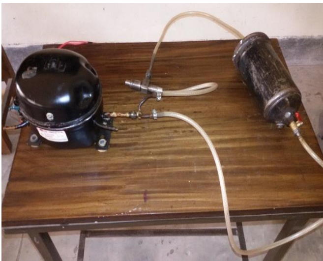
(a) MQL set up (b) Operation performing on MQL
