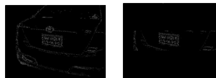
Fig.2 : (a) Sobel vertical edge detection (b) Effect of threshold
