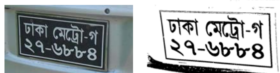
Fig.3 : (a) Extracted Candidate plate (b) After Inverting and threshold
