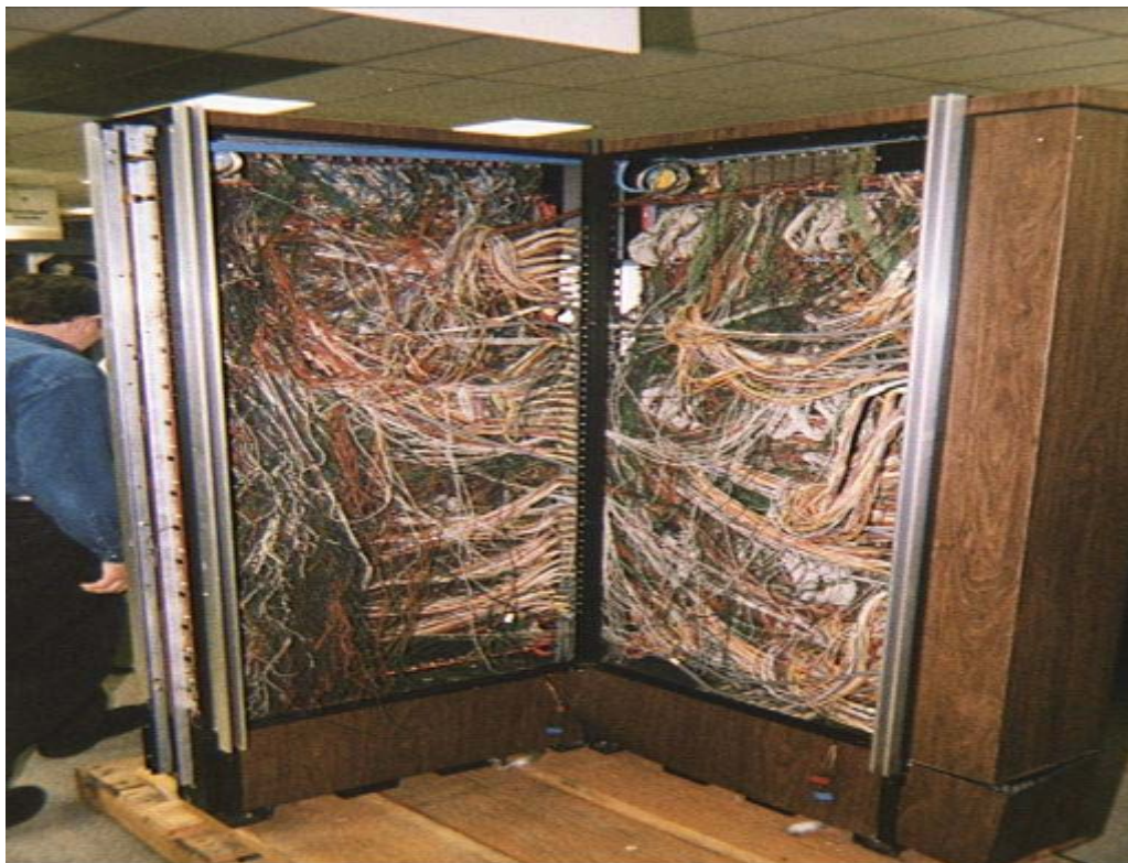
Fig.15 : Typical wiring of an early mainframe computer [photo courtesy: The computer museum]
