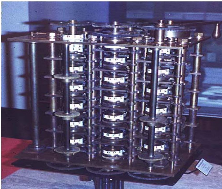
Fig. 11 : Babbage's Difference Engine [photo 2002 IEEE]
