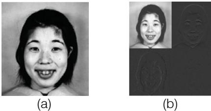
Fig. 1 : (a) Sample image from JAFFE database (b) 2-D Wavelet transformed image at level 1
