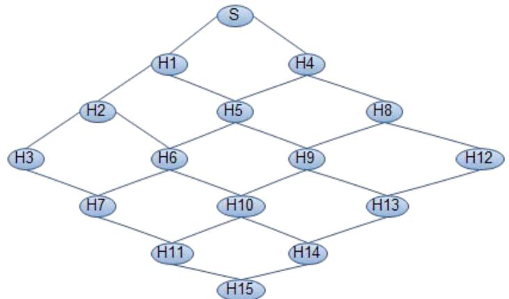
Fig. 2 : Mesh Representation of example multicast model
