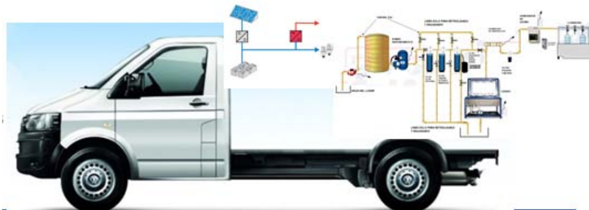
Diagram 11 : Proposed water purification system photovoltaic and transportable
