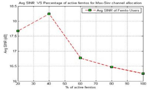
Figure 4 : Average SINR Vs Percentage of active femtos for Max-SINR channel allocation
