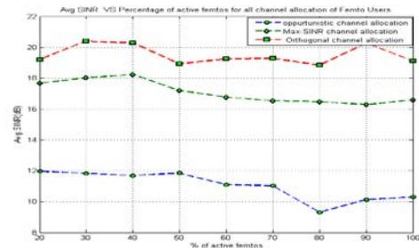
Figure 5 : Comparative analysis of Average SINR experienced by Femto Users varying the percentage of active femtos for the three channel allocation schemes
