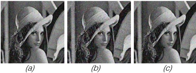
**Fig. 5** Watermarked image corrupted by different noises (a) Gaussian noise (10%) (b) Salt and pepper noise (10%) (c) Poisson noise (10%)
