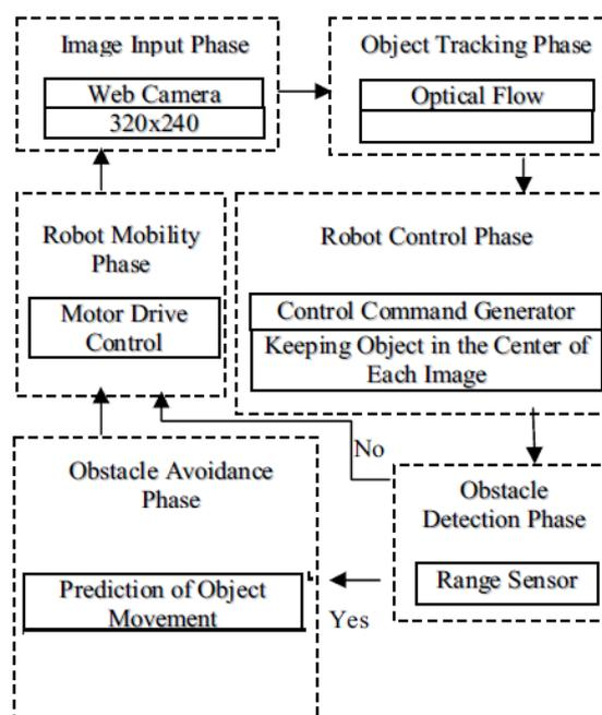
Figure 1: This block diagram shows the overall system
