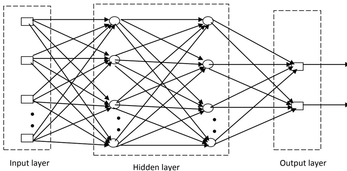
Figure 1: Structure of the artificial neural network with Double hidden layer
