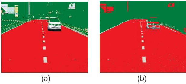
Fig.7 : Labeling image (a) and output taking width as an attribute (b)
