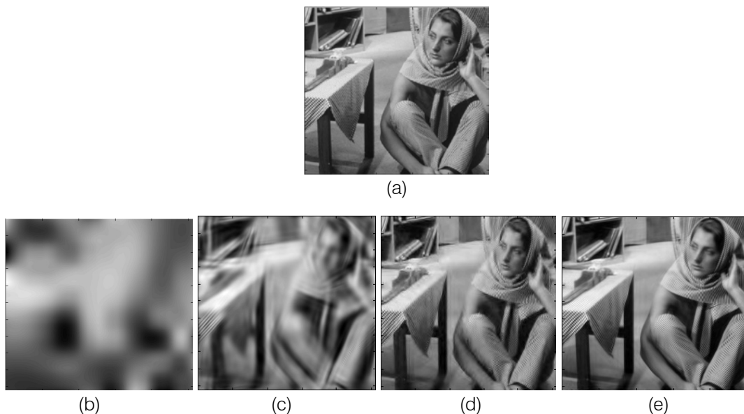
Fig. 3: Barbara image for compression ratio of 1:20 (a) Original image (b) Wavelet with existing quantizer (c) Curvelet with existing quantizer (d) Wavelet with proposed quantizer (e) Curvelet with proposed quantizer
