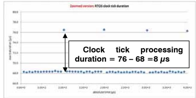
Figure 2 : Clock tick processing duration of the baremachine-zoomed
