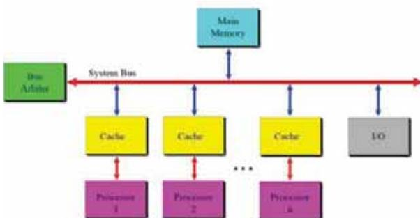
The hardware platform used for this evaluation is a Symmetric Multiprocessing (SMP) system with four identical processors connected to a single shared main memory using a system bus. They have full access to all I/O devices and are treated equally.
