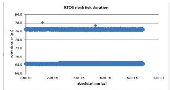
Figure 3 : Clock tick processing duration of the baremachine
