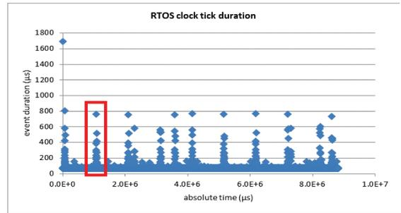
Figure 6 : Clock tick duration test for Enlightened VM in scenario 1
