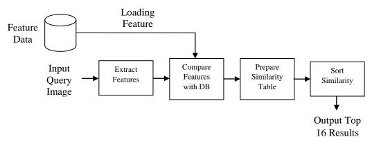
Figure 3.2 : Block Diagram of Image Retrieval
