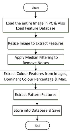
Figure 3.3 : Flow char of feature database preparation
