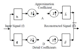
Figure 5 : 1-D wavelet analysis and synthesis filter
