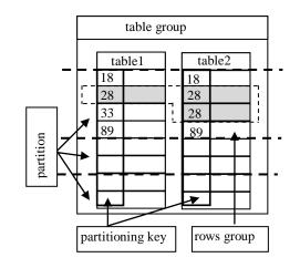
Figure 2 : Data model for relational cloud database
