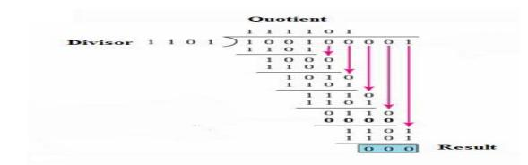
Figure 8 : CRC in receiver side
