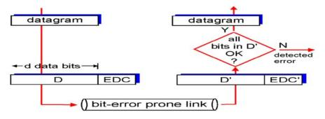
Figure 5 : Error Detection Mechanism
