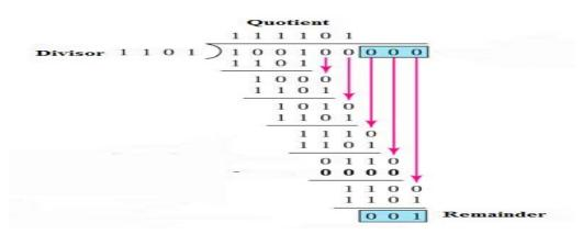
Figure 7 : CRC in sender side
