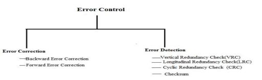
Figure 2 : Error Control Methodologies
