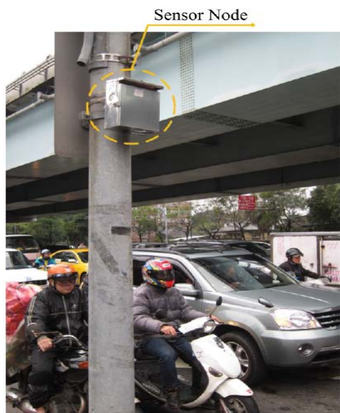
Figure 11: Deployment of the air quality monitoring system. A sensor node was attached to the traffic signal pole
