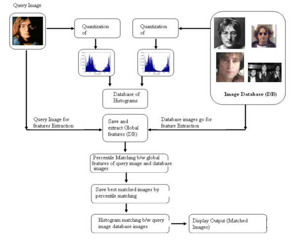
Figure 4 : Block Diagram of Proposed CBIR System
