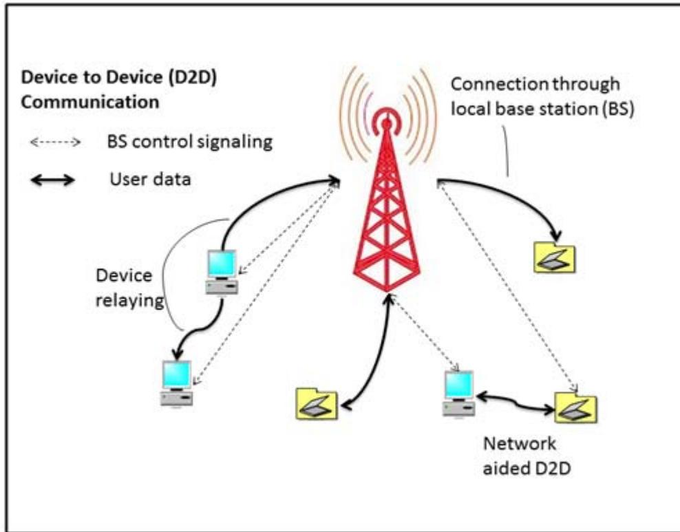
Figure 1 : Architecture of envisioned D2D omunication
