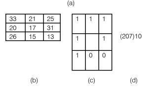
*Figure 2:* Multi Region-Local Binary Pattern Code generation (a) Division of Region of size 9\*9 into '9' sub regions of 3\*3 (b) Representation of average values of '9' sub region of 3\*3 (c) MR-LBP Representation (d) MR-LBP Code.
