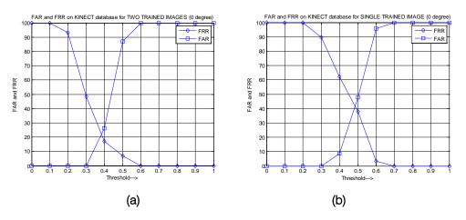
Fig. 7 : Threshold versus FAR & FRR on Kinect database for (a) One & (b) Two trained images
