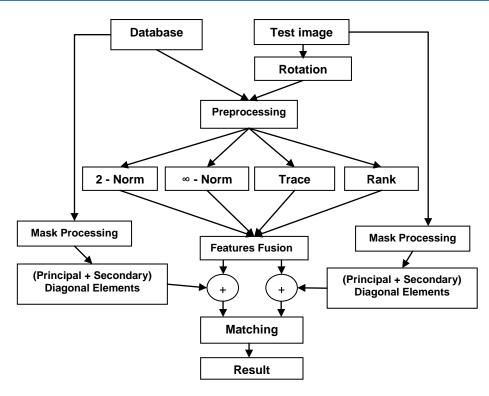
Fig. 1: Block diagram of the Proposed FR DMF model
