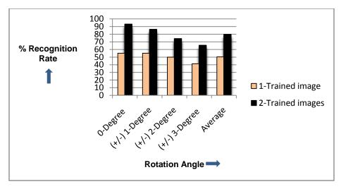
Fig. 8: Comparison of Maximum % RR for Different Rotation Angles on Kinect database
