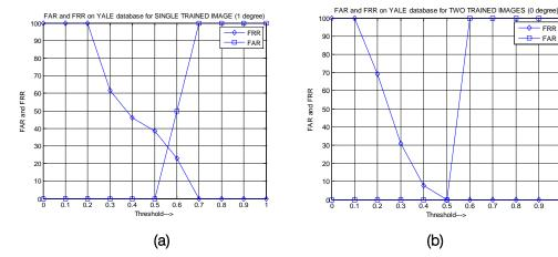
Fig. 5: Threshold versus FAR & FRR on Yale database for (a) One & (b) Two trained –images
