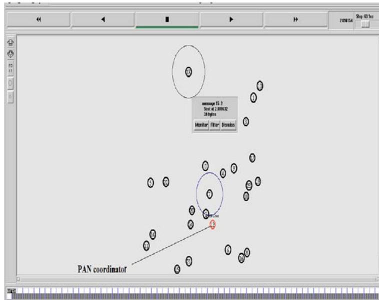
Figure 2: Initial nodes movements before the nodes associates with its coordinator at time 2 sec
