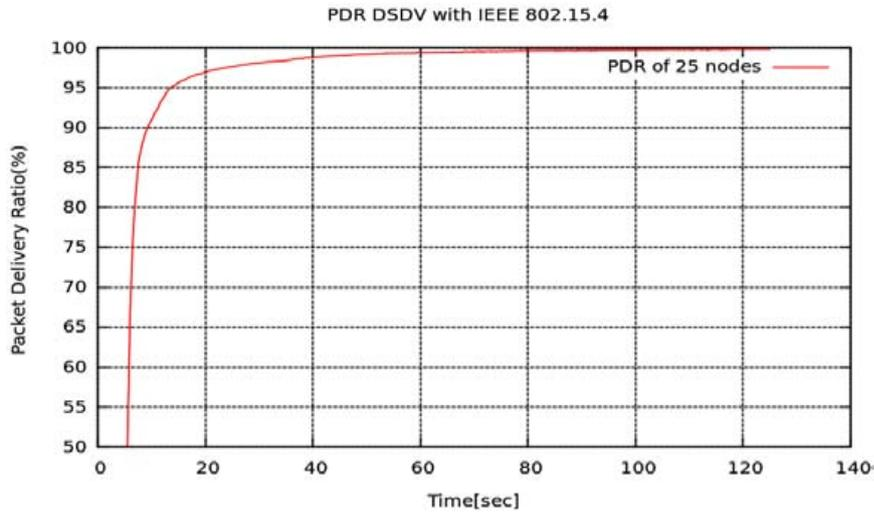
Figure 6: Packet delivery ratio vs simulation time
