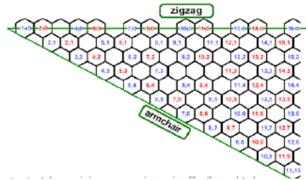
Figure 12: Single Walled Carbon Nanotubes (Graphene) Sheet with the possible rolling designs (Zigzag and Armchair)
