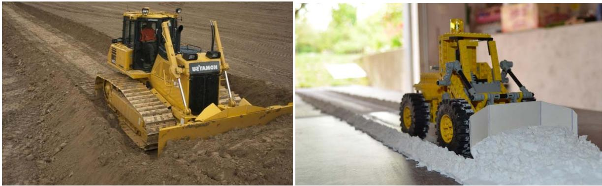
Figure 3: Side dump happening on the side of blade.
