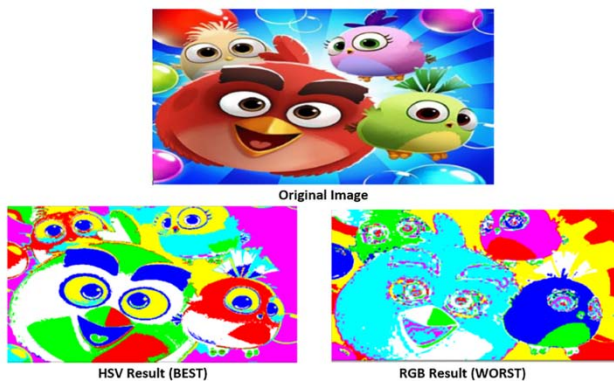
Figure 15: HSV Result on Bird image after Color Segmentation
