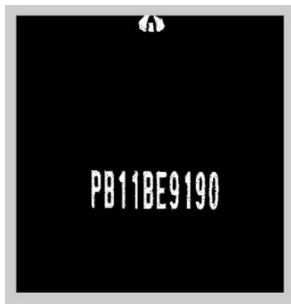
Fig. 8: Preprocessed Image after plate localization in SVM Classifier.
