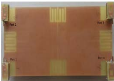
Fig. 1: Multiband MIMO with Insertion of parasitic element [9].
