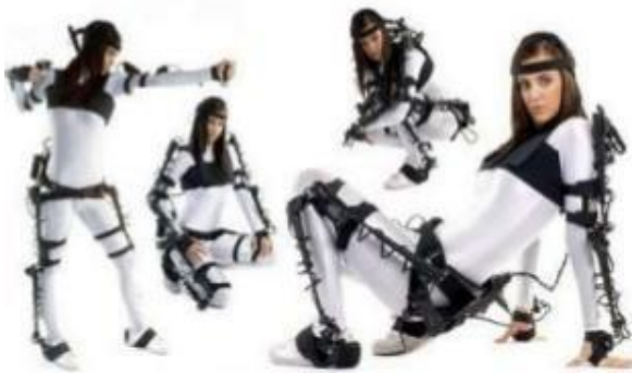
Fig. 3.1: Mechanical Motion Capture using Exo skeleton
