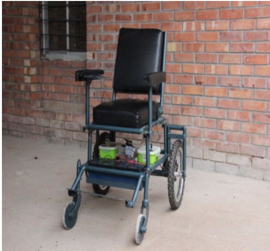
Fig. 8: Android controlled smart wheelchair for disabilities.
