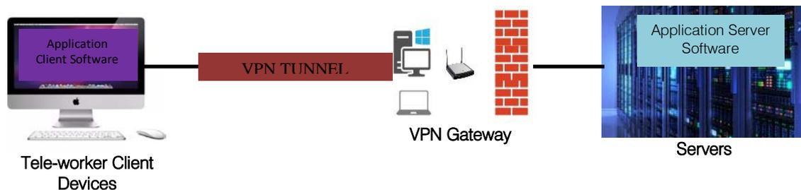
Figure 2: Tunneling Architecture
