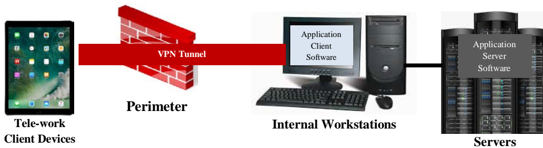
Figure 4: Remote Desktop Access Architecture
