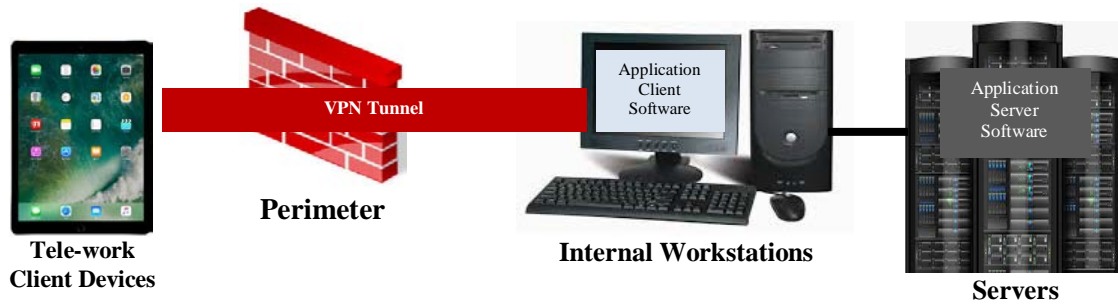
Figure 5: Direct Application Access Architecture
