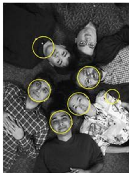
Fig. 1: Face detection with the latest method [12]; The algorithm is unable to detect a few rotated faces.
