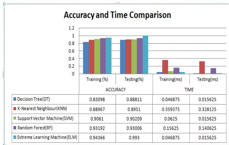
*Figure 8:* Accuracy and Time Comparison
