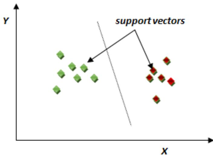
*Figure 2:* Support Vector Machine Classification
