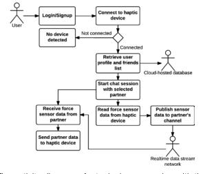
Fig. 5: The activity diagram of a typical user session with the haptic
