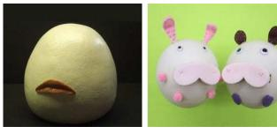
Fig. 3: Left: first version of Kissenger was a headshaped device with a realistic pair of lips. Right: second version of Kissenger was designed to look like a cute animal character with soft silicone lips.
