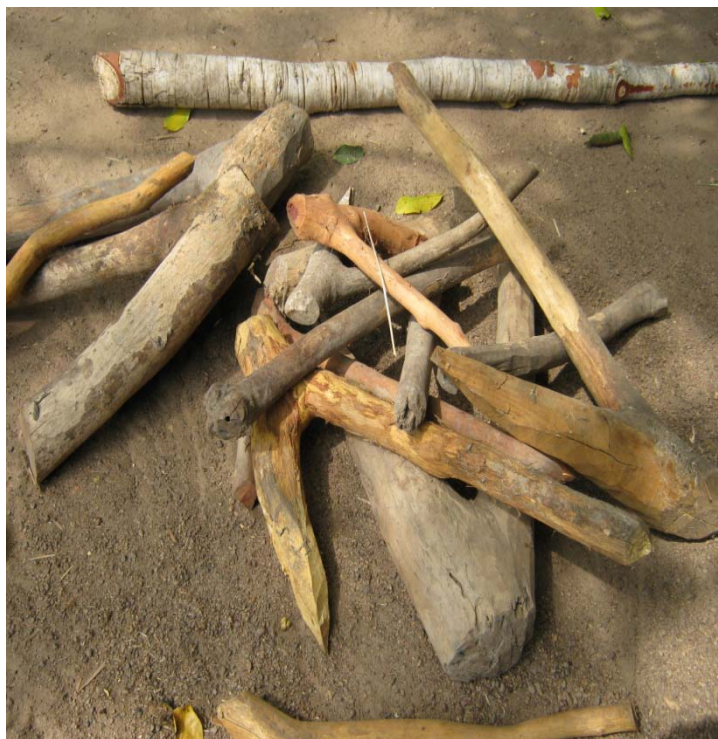
Plate IX: Different sizes of agbe (hoe handles) from different tree species under different stages of completion
