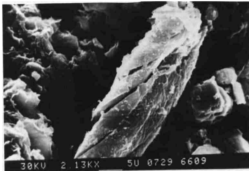
Picture 1: SEM photo from area 26. Quartz crystal having suffered a shear stress, surrounded by flakes of montmorillonite. Magnification x 2000.
