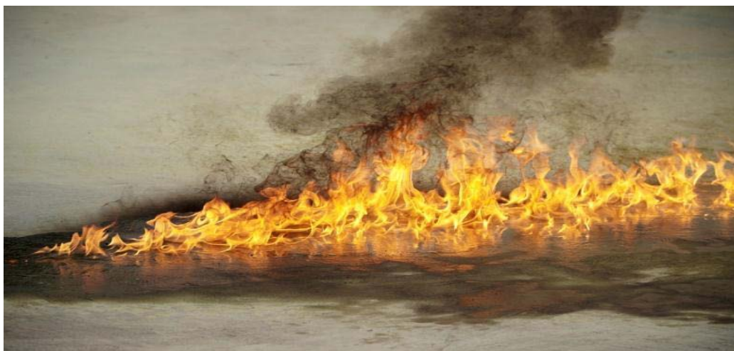
Figure 13: In Situ Burning of Spilled Oil
