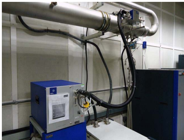
Figure 13: PNC installed in the CVS dilution tunnel.
