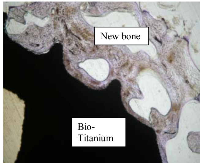
Figure 4 : Electron microscope: bone/biotitanium active interface
