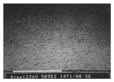
*Figure 4 :* Scanning electron micrograph with high resolution (X503) of the surface of a titanium dioxide-blasted threaded implant (Astra Tech TiO-blast)
