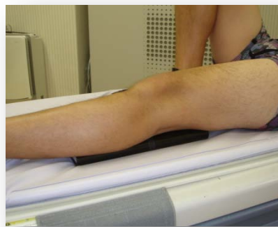
Fig. 1 : The phantom(Taisho-Toyama Pharm. Co., Ltd, Tokyo. Japan) consisting of a cylinder composed of a material corresponding to cortical bone and filled with a material having a bone density corresponding to cancellous bone was placed under the knee.
