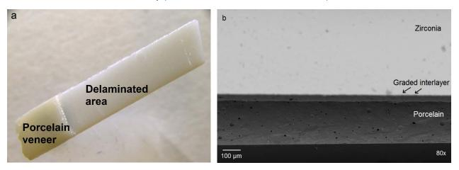
*Figure 4:* (a) Stereo microscope image of a fractured specimen: specimen from G1 exhibiting extensive delaminated area of veneering porcelain. (b) Representative side view SEM micrograph image showing tested sample from G2.
