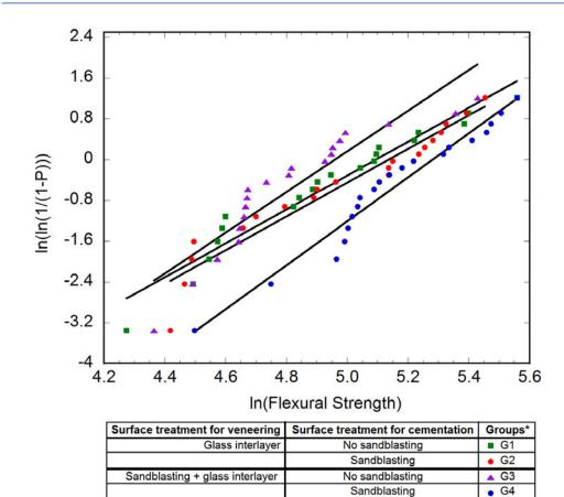
*Figure 3:* Weibull plot of tested groups. The similar slope of the curve fits (black lines) indicates similar strength reliability (similar Weibull modulus; 3.31<m<4.31).
