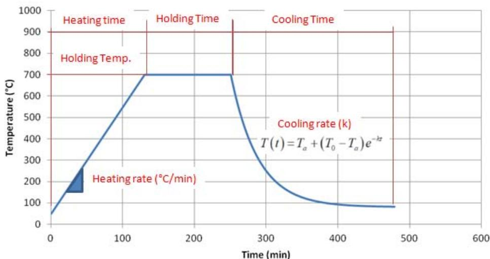
Figure 2: Illustration of sintering temperature curves and control factors: Holding Temperature ( $T_{hold}$ ), holding time ( $t_{hold}$ ), cooling rate (k) and heating rate (Hr)
