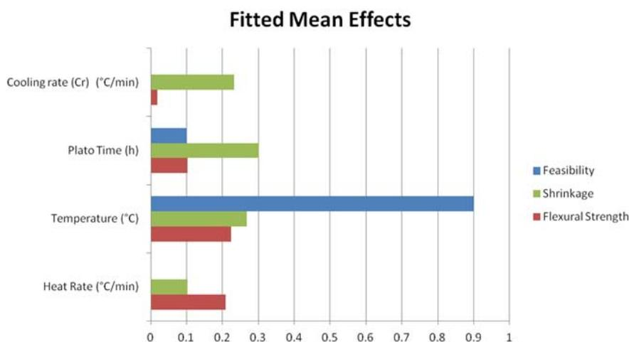
Figure 3: Main effect of control parameter on feasibility, flexural strength and shrinkage
