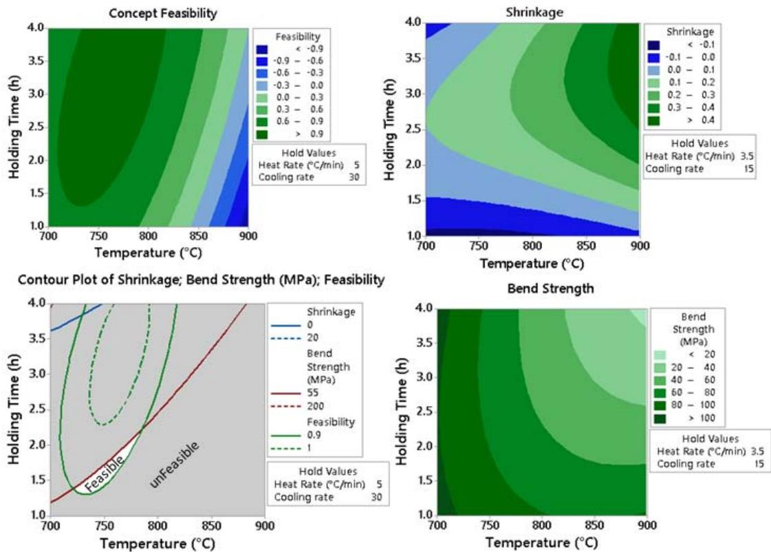
Figure 7: Contour diagrams of Flexural strength, feasibility, shrinkage and the overlap diagram with combination of high values
