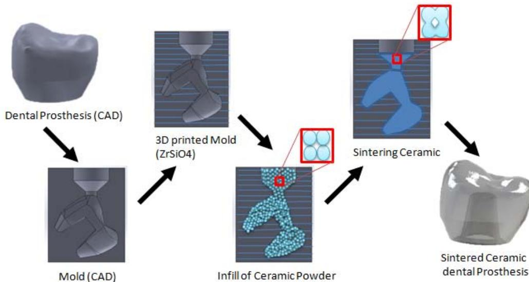
Figure 1: Schematic of ceramic dental prostheses based on ZrSiO<sub>4</sub> – Glass composites fabricated by indirect Additive manufacturing
