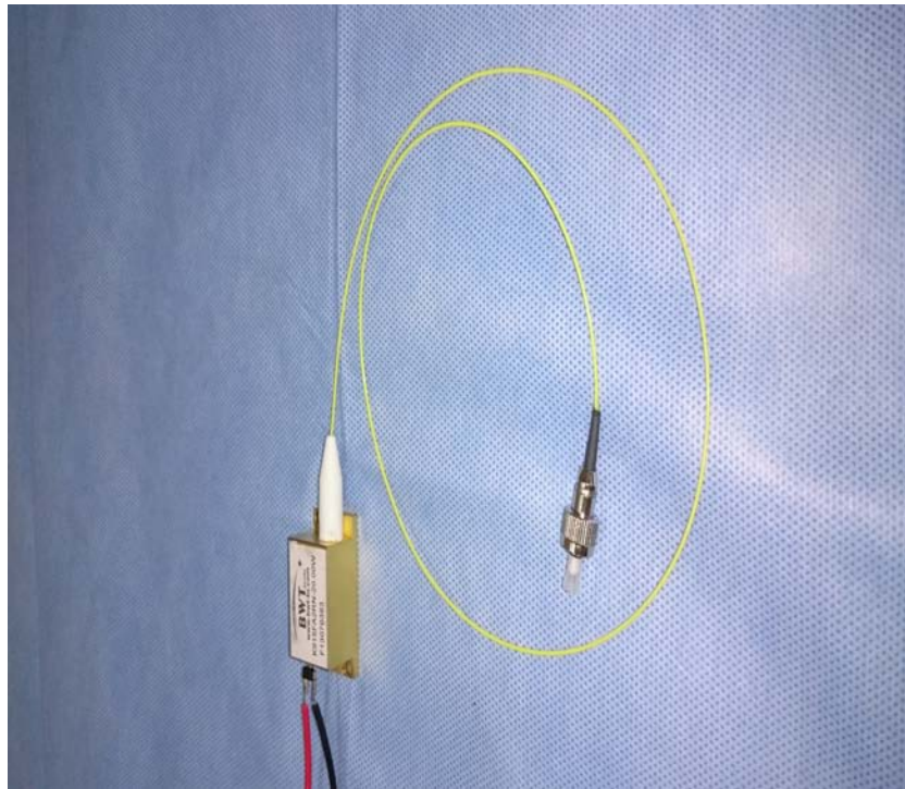
Photo 3: Laser diode coupled with 0.1 mm optical fiber
