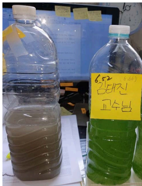
Figure 8: After treatment without growth of HAB (Left) and before treatment with growth of HAB (Right) of H_2S bubbling
