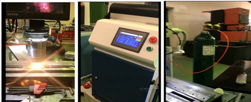
Fig. 1: Show the Pulse Nd: YAG laser welding system, (a) laser welding machine ; (b) laser generating device and (c) argon gas tube
