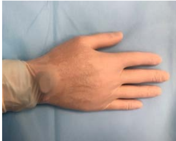
Figure 3: Individual dosimeter fixed in the area of the wrist joint
