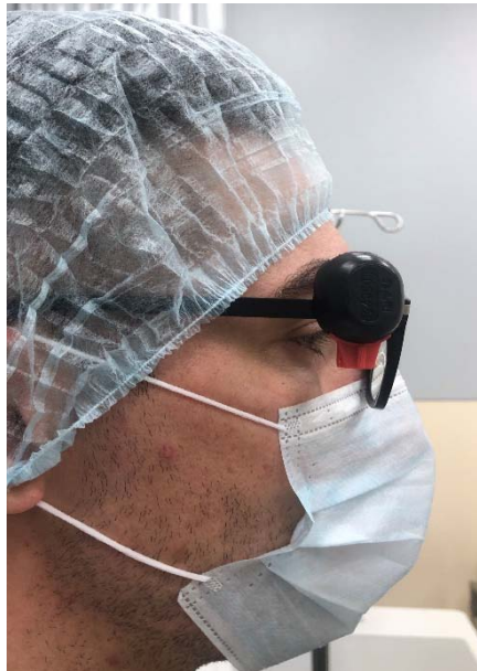
Figure 1: Individual dosimeter fixed in the orbit area
