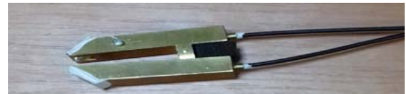
Fig. 2: A clip through which a probing beam of light with an adjustable wavelength passes
