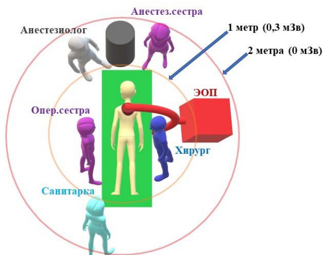
Figure 7: Scheme of x-ray radiation spreading in the operating room
