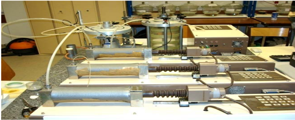
Fig. 7. Triaxial cell of type Bishop-Wesley revolution controlled with three pressure-volume controllers
